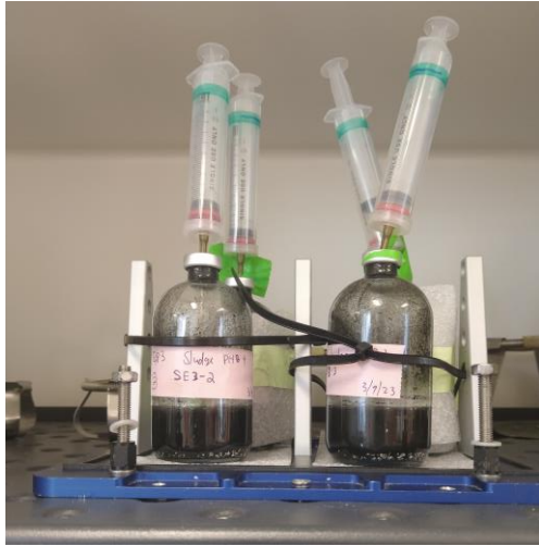
Figure 2: Experimental microcosm setup with liquid samples from SVCW.
